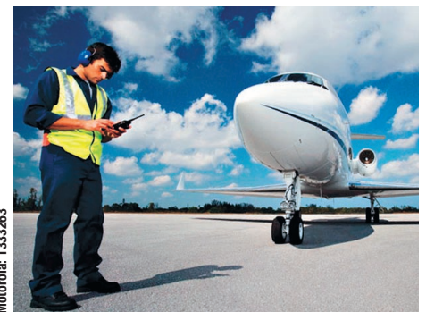
■ Motorola’s MTC 100 is a Windows Mobile PDA that has WiFi as well as Tetra. It supports context-aware security applications through Tetra or WiFi, depending on which is available at the time. Appear plans to use it in a number of its implementations.
